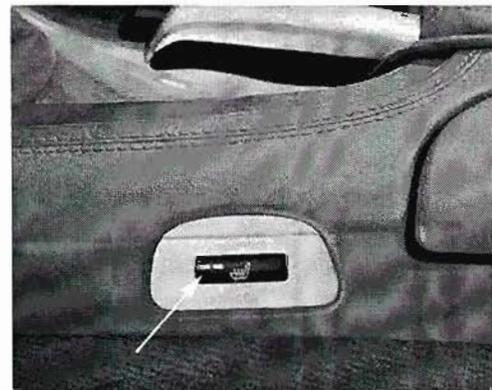
The two position Seat Heater Switches are located on the left and right sides of the center console as shown above.
