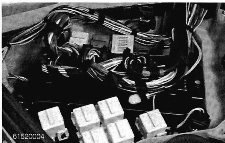
The E box is shown above containing the traditional engine fuses.
