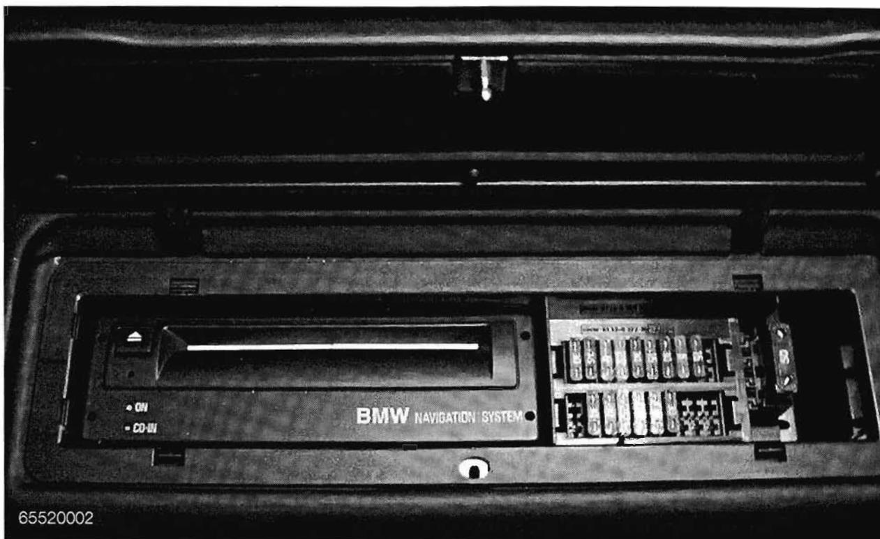
There are additional vehicle fuses located in the Navigation cd storage compartment.
