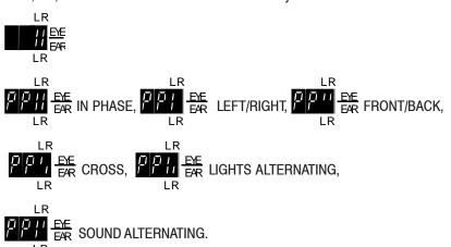
In dbb and dSb tone PHASE controls which eyes are on at the same time, and also the sound generator #2 controls.
